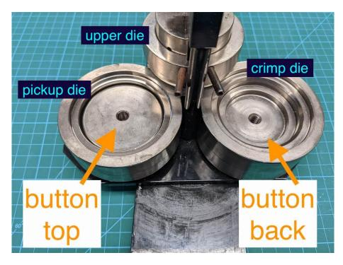
5) Place the top shell in the pickup die with the completely flat surface facing up. Then, place the paper image on top, lastly the mylar sheet. Think of it like a sandwich!
