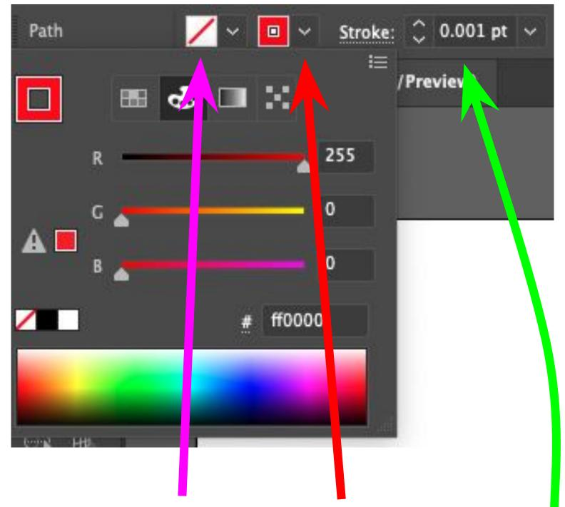
8. Change the Fill to "none", the Stroke to "red" (it must be absolute red, rgb(255, 0, 0), #ff0000), and the Stroke Width to ".001" (points or inches).
